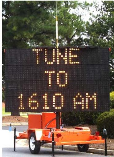
**Figure 3: Portable Dynamic Message Signs with Highway Advisory Radio**
